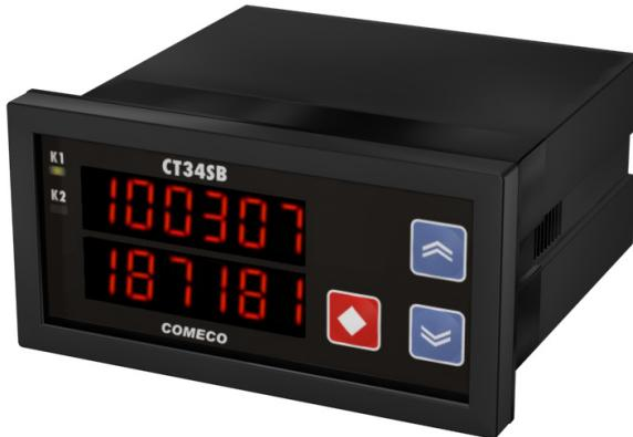
Counter software allows a convenient programmable scaling of both measured flow signals and applying various calculations on both flow rates. CT34SB is equipped with two 6-digit LED displays indicating current flow-rates, mathematically calculated values as well as accumulated total counts. The counter has also an optional relay output for generating impulse when certain total value is reached (dosing function).
